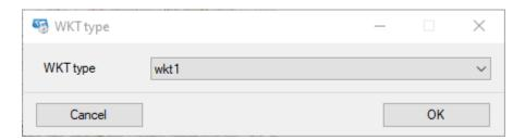
For each existing vectorial theme, four files will be created, according to ESRI standards, with the extension .shp, .dbf, .shx and .prj (containing the WKT specifications).
