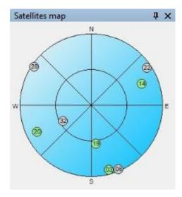
A sky map appears with the location of the satellites. Each satellite is represented by a colored dot with the number of the satellite inside. The meaning of the colors is as follows:
