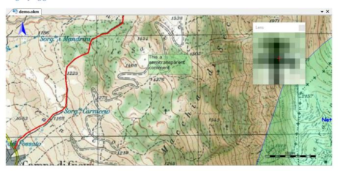
The lens windows displays a strong magnification of the map image around the mouse pointer. It can only be displayed for raster or web maps.
