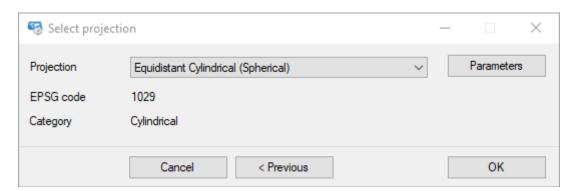
If the desired projection does not appear in the list and the map surface covers a small region, we can obtain a fair approximation by selecting the *Equidistant Cylindrical (Spherical)* projection.
