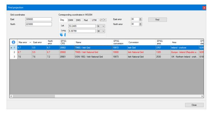
The metric coordinates of a grid intersection and the WGS84 geographic coordinates of the same point taken, for example, with Google Earth must be indicated.
