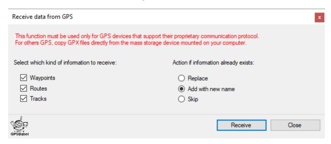
You can specify which types of GPX data you want to receive from the GPS:
