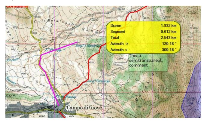
To activate the distance calculation function, use the *Home - Tools - Distance* menu; click with the left mouse button on the map to indicate the starting point; then indicate, by the same method, the intermediate points and the end point.
