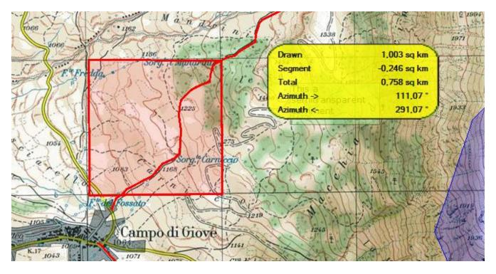
To activate the area calculation function, use the *Home - Tools - Area* menu; click with the left mouse button on the map to indicate the first node of the polygon; then indicate, with the same method, the remaining nodes of the polygon.
