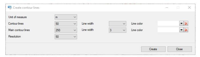
Select the unit of measurement and the distance between the contour lines you want to draw. It is possible to specify the interval of the main contour lines in order to indicate different graphic attributes (line thickness and stroke color).
